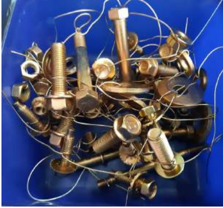
Stripped, tied, dipped, and coated
